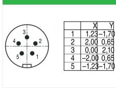
Contact arrangement (Plug-in side)
